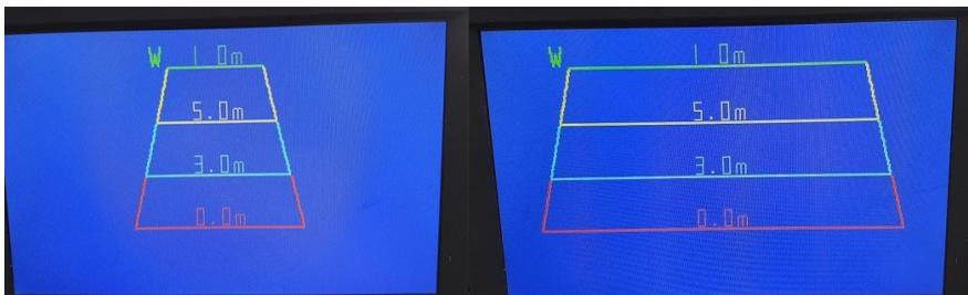
To adjust the values on the lines, go back to the main park setup menu and enter the line number menu. To modify values use the up and down keys to change the number to the required value and the Menu button to go to the next number to adjust.
